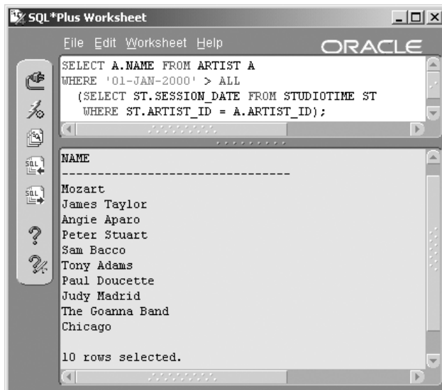
Figure 12.12 Values Can Be Passed from a Calling Query into a Correlated Subquery.
